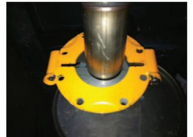
approximate gap of 12-15mm between the 2 clamps. The bolts will be tightened properly later on in the fitting process. Do the same for the second set of clamps at the other end of the catalytic converter.
